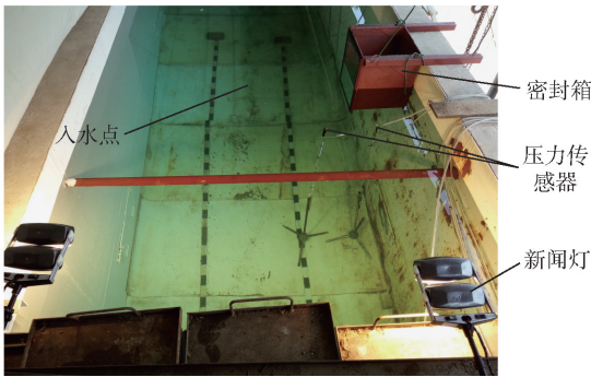
图 2 试验系统实物图 (视角为弹道终点指向发射点) Fig. 2 Photo of experimental system (the visual direction is from the ballistic end to the launch point)
